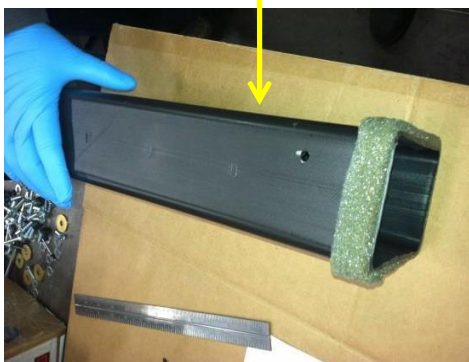
Top of duct as it is installed in the truck
