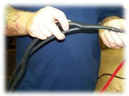
Assemble the refrigerant hoses, drain 17 tube, power cable assembly and condenser wiring harness through the provided flanged grommet. Make sure you have the correct end of the condenser harness and refrigerant lines going inside the cab.
