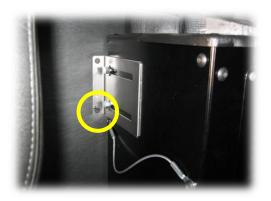
After the brackets are secure, reinstall the upholstery. Make sure the unit is firm against the rear wall of the cab and tighten the bolts on the side of the unit.
