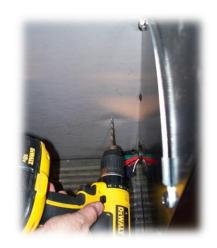
Using the locator hole, carefully drill a 3 inch hole through the rear cab wall. USE CAUTION: There could be hidden wires. Do not drill completely through the upholstery without checking first!
