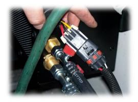
Now, secure all hoses, wires and cables with cable ties.
