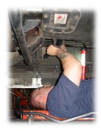
Attach Cables to Truck Batteries
