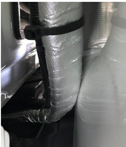
Figure 1.20: Hose Rub (NOT ACCEPTABLE)
