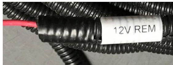
Figure 2.4: 12 V Remote Branch of Vehicle Harness
