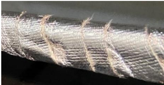
Figure 1.7: Hoses Wrapped in Heat Shield Tape
