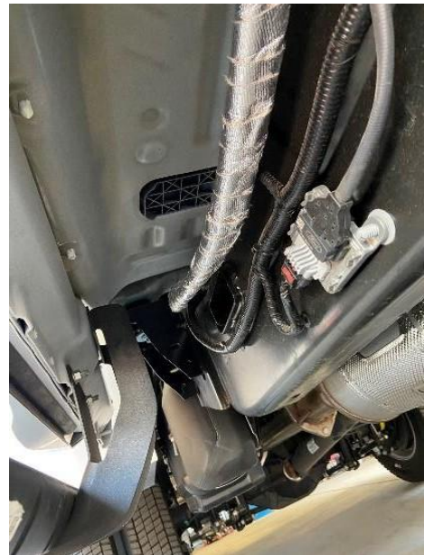
Figure 1.9: Hoses Routed Under Vehicle
