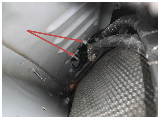
Figure 1.7: Bolts that require removal
