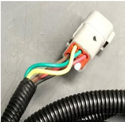
Figure 2.3: 6-way Deutsch Branch
