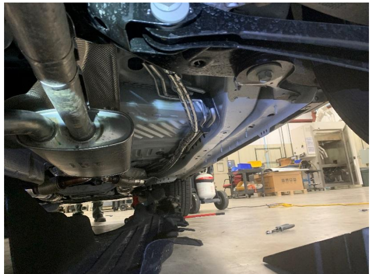
Figure 1.9: Hoses Routed Under Vehicle
