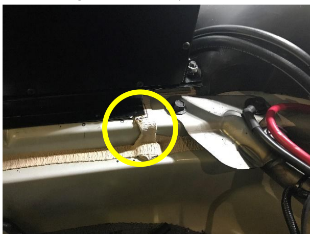
Figure 1.6: Portion of Seam Sealer to Remove
