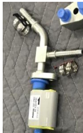
Figure 1.13: Discharge Line Alteration on 2021-2022 Tahoe
