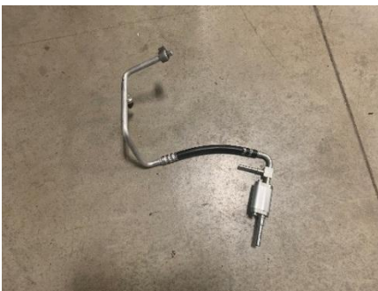
Figure 1.13: Discharge Line Alteration on 2021-2022 Tahoe
