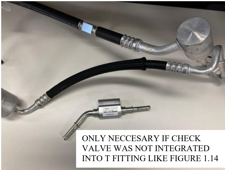
Figure 1.15: Check Valve Alteration for non-integrated check valve
