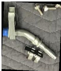
Figure 1.13: Discharge Line Alteration on 2021-2022 Tahoe
