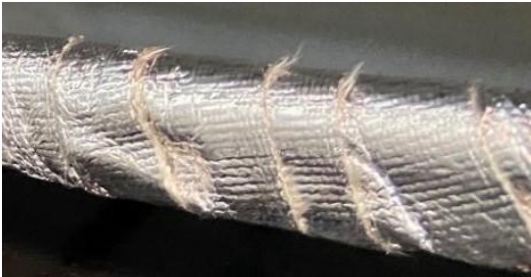
Figure 1.5: Hoses Wrapped in Heat Shield Tape
