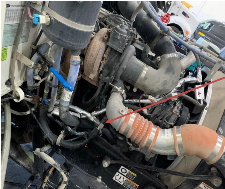
Figure 1.9: Suction Line Alteration
