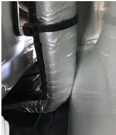
Figure 1.19: Hose Rub (NOT ACCEPTABLE)
