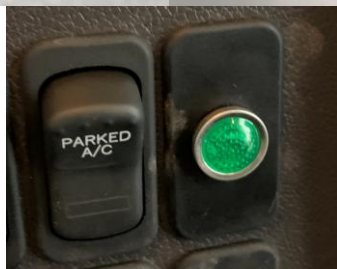
Figure 2.9: Rocker Switch, Harness Connection, and Completed Install Cosmetic
