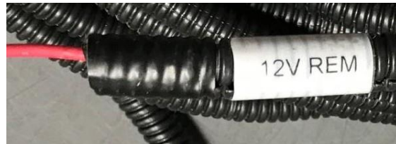
Figure 2.4: 12 V Remote Branch of Vehicle Harness
