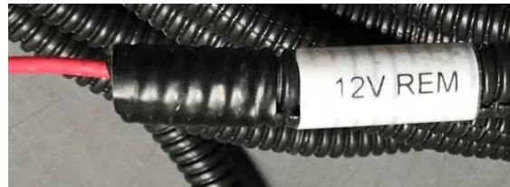
Figure 2.4: 12 V Remote Branch of Vehicle Harness
