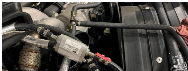
Figure 1.12: Example CV in Discharge Hose
