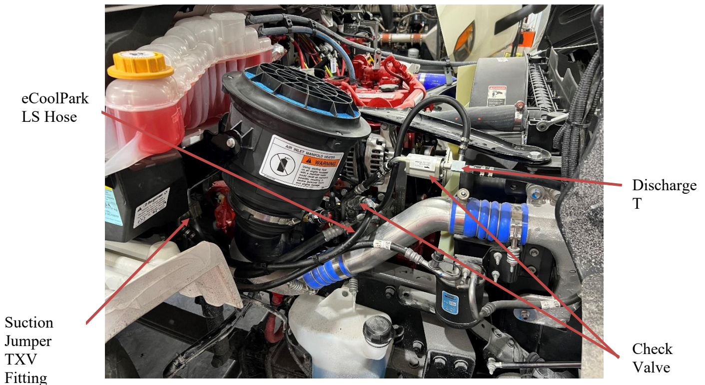
Figure 1.13: Finished A/C Hose Alteration
