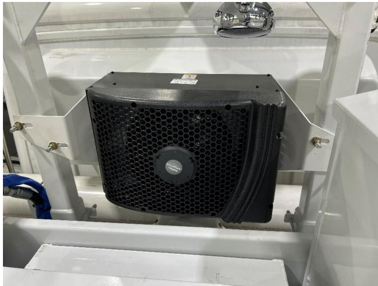
Figure 1.4: eCoolPark 1.5 Mounting Examples
