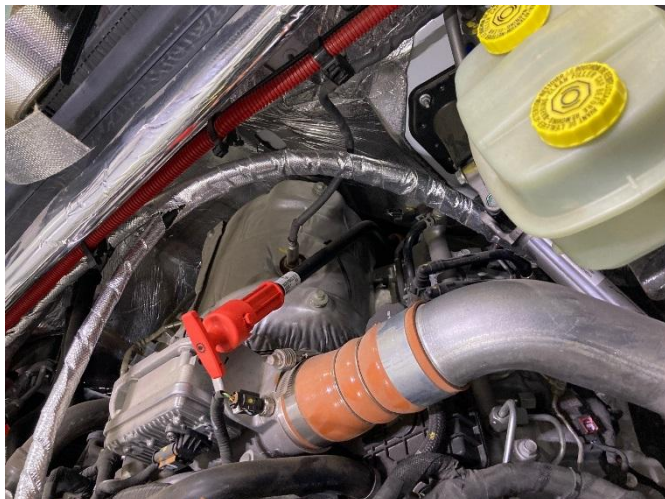
Figure 1.6: Hoses Routed into Engine Bay
