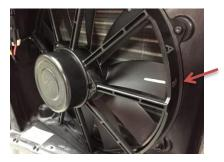
7. Rotate clockwise 1 cogging torque position and mark the third test location "C".
