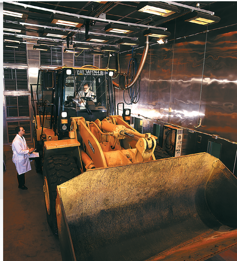
Extremes in temperature, humidity, wind velocity, and sun load are duplicated in the full size environmental chamber to validate performance of Bergstrom's cab climate systems.
